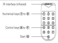
The data transmission to and from the sensor is ensured by an IR interface. The <u>connection</u> between the remote control and the sensor can only be established when the sensor is in <u>configuration mode</u>.
