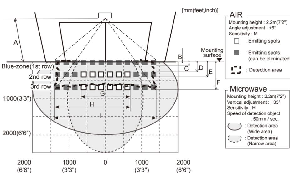
**NOTE** The actual detection area may become smaller depending on the ambient light, the color / material of the object or the floor as well as the entry speed of the object. The sensor may not be activated when the entering speed of the object or a person is slower than 50mm / sec. or faster than 1500mm / sec.
