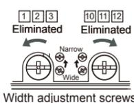
**NOTE** When setting the detection area width, make sure to turn the adjustment screws until it clicks. **1 2 3** cannot be eliminated separately, neither can **10 11 12**.
