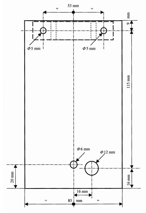
5 mm hole diameter6 mm hole diameter12 mm hole diameter
